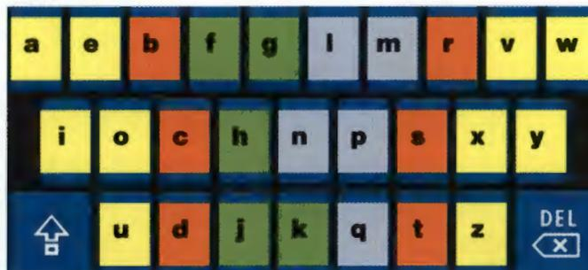
*Finally*, the AEIOU Technical Drawing is a depiction of a black physical keyboard with standard layout (akin to a QWERTY<sup>1</sup> keyboard) for all non-letter elements in white, and with the letters arranged, in reading order from left to right and top to bottom, as: AEBFGLMRVW IOCHNPSXY UDKQTZ. The AEIOU Technical Drawing is depicted as follows:
