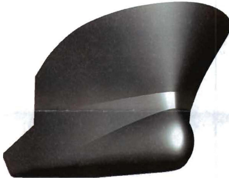
Figure 2: Bulbous Bow 3D Model
